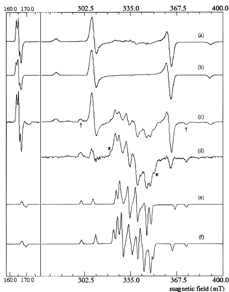
Figure 1. Experimental ( \nu = 9.434 GHz) and computer-simulated EPR spectra obtained from the bis-azoalkane 2(N_2)_2 in MTHF glass at 77 K. (a) Spectrum obtained on multiline UV irradiation (333, 351, and 364 nm) assigned to the triplet biradical 2(N_2) . (b) Simulation for a triplet state using the spin Hamiltonian in eq 1 with g = 2.002 . (c) Spectrum obtained on monochromatic 333-nm irradiation assigned to a mixture of the triplet biradical 2(N_2) and the quintet tetradical 2 . (d) Difference spectrum [Figure 1c - 1.337 \times Figure 1a] for removal of contributions from triplet 2(N_2) . (e) Simulation for a quintet state using the spin Hamiltonian in eq 1 with g = 2.003 . (f) Simulation for a quintet state using the spin Hamiltonian in eq 2 with g = 2.003 .
